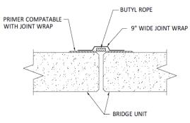
NOTE: Joint is considered "soil-tight". Additional protection is recommended if a water-tight joint is required.
